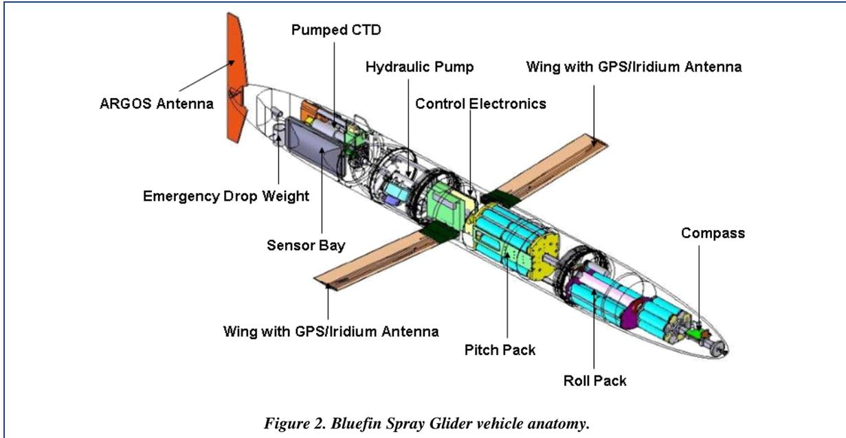
An integrated GPS and Iridium antenna is installed in each of the vehicle's wings. The wings are bolted onto the pressure housing at mounting holes in the side of the housing and use a bore seal O-ring to provide a sealed volume inside the pressure housing. Antenna cables are passed through the mounting holes within the circumference of the bore seal. The vehicle's wings provide stability during the glide, and work to change heading during a roll.
