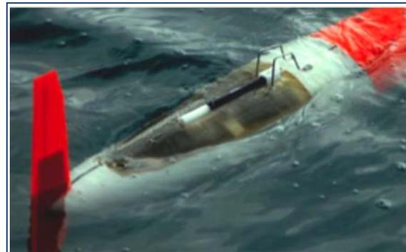
*Figure 4. The Spray Glider's free-flooded sensor bay.*
